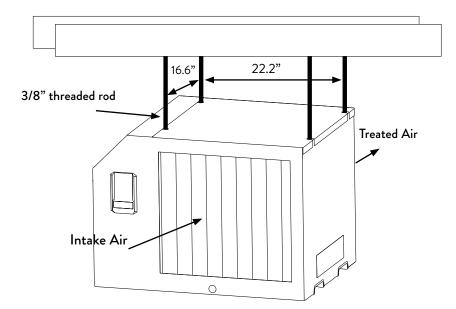
Threaded rods should be engaged no less than 2" into machine.
